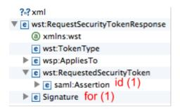
Most of the attacks demonstrated in Somorovsky and others' paper are possible because the application validating SAML token fails to properly and unambigously handle the token structure. The implementors make a number of assumptions, for example that the token will be always properly formed XML document, compliant with the SAML schema and with properly linked references.
